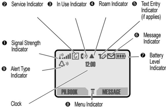
**1 Signal Strength Indicator:** Shows the strength of your phone's connection with the network.
